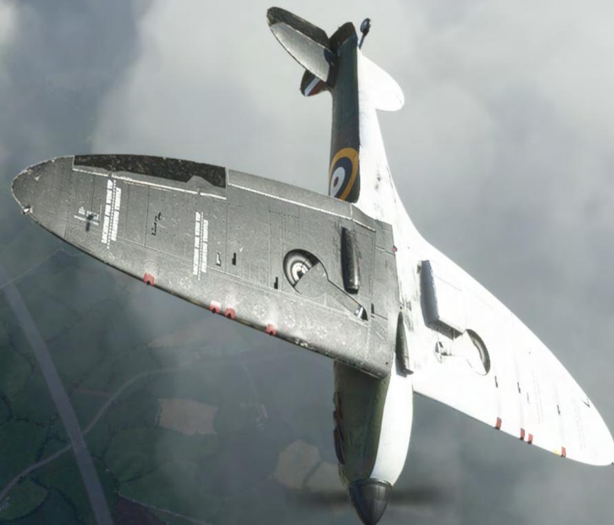
In the very early stages of WWII, the RAF used a "DayNight" black and white scheme for the undersides of their fighters. N3200 "QV" carries an example of this scheme. It was not long, however, before all fighter schemes were standardised with an underside painted in "sky" or duck-egg green/blue
