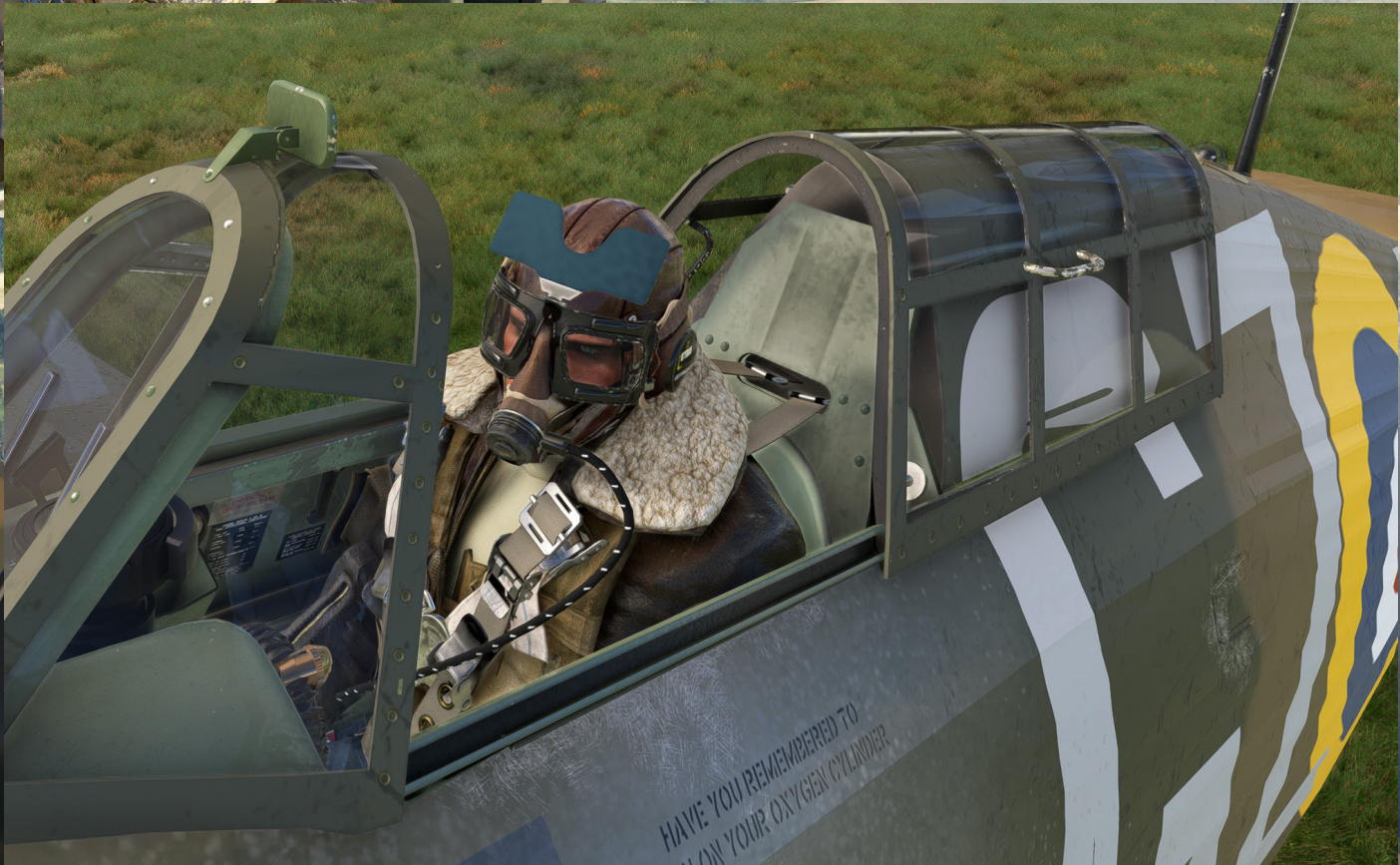
This is the early 1938 pattern goggles and oxygen mask. A swing-down sun-shade was provided for the goggles. This cumbersome outfit was soon replaced with lighter, smaller goggles although the side entry oxygen pipe remained for some time. Clicking the oxygen supply socket (49) toggles the mask and goggles for the pilot.
